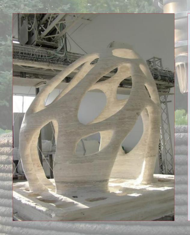
The technology works by depositing alternating layers of Powder of granular matter like sand or aggregate, and specially formulated binding "ink" that fuses the grains together. This enables printing of solid structures from the ground up, wall by wall, layer by layer
