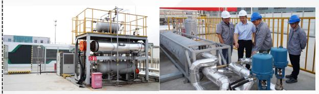
Mg-based solid-state hydrogen storage tank and its test system
