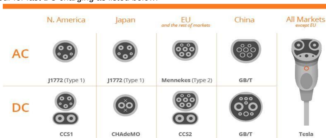
Fig.No.39 Types of Charging Plugs or Connectors (Source: EnelX) [10]
